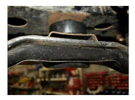
Use the 3 x 25mm x 20mm (8.5mm ID) Round Spacer – Steel (D) on the front mounting holes of the metal skid plate.
