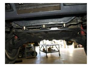
Use the 2 x 30mm x 21mm (9.5mm ID) Round Spacer – Nylon (E) on side mounting holes of the metal skid plate.
