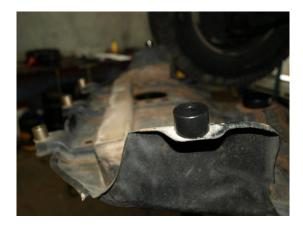
For these five locations use the supplied M8xP1.25 x 40mm Bolts (H) and M8 Flat Washers (I) – and on the front three spacers also use the M8 Split Washers (J).
