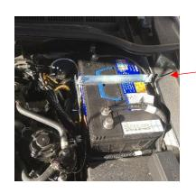
6. Place J hooks in the holes in tray, lower battery in and place hold down bracket on and tighten down until the battery is firm.
