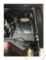
4. Remove clip on sedimenter wire and refit to tray
