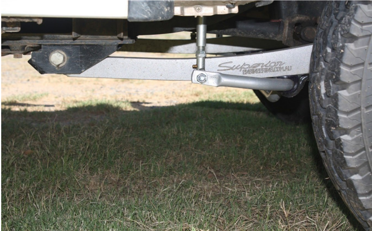
Image 3: HYBRID ARM FITTED CORRECTLY without abs lines
