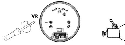
Use the VR roll, which is enclosed in our accessory pack, to adjust to the accurate SPEED.
