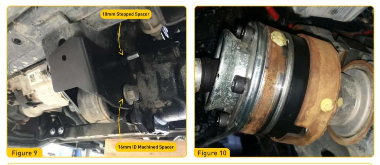
10. Once all components have been installed in the prescribed order, tighten all bolts to recommended torque values and reinstall the bash plates. Now that you have lowered the front diff mount, the bash plates will require spacing or modification. Spacers for bash plate relocation are not included in the kit. Spacer requirements are specific to the bash plate brand and design. The Roadsafe Bash Plates do not require modifications or spacers to be fitted with this diff drop kit.
