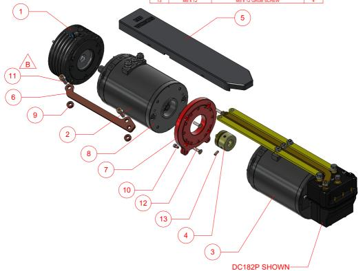
When the winch is not in use, springs apply pressure to a steel disc, which in turn presses against the brake disc and its friction material. This engages the brake, preventing the winch drum from turning under load or unintentionally spooling out the rope.
