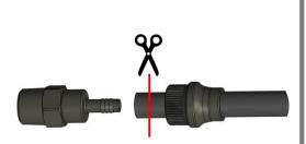
The hose may be shortened by unscrewing sleeve and sliding sleeve back. Remove hose from barb and cut hose using sharp razor blade. Push barb into hose and screw sleeve onto barb fitting.
